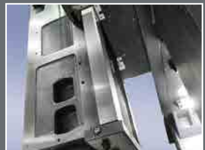
■ Hardened and Ground Box Guideway on Z-axis (DCV2012B)
