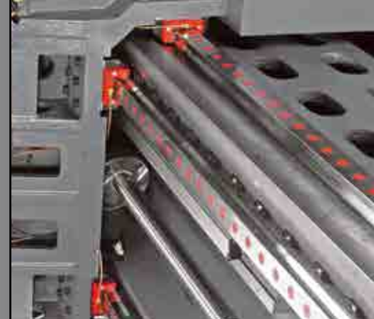
■ Horizontal and Vertical Support of the Headstock
