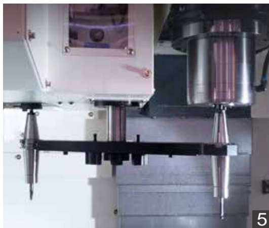
| 4. 24T for disk type tool magazine | 5. Auto tool change time (T-T): 1.8 sec. | | 6. Absolute encoder ATC system |
