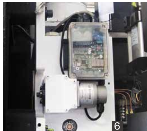
| 4. 24T for disk type tool magazine | 5. Auto tool change time (T-T): 1.8 sec. | | 6. Absolute encoder ATC system |
