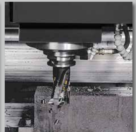
● Optimal Chip Removal (50#) End Milling
