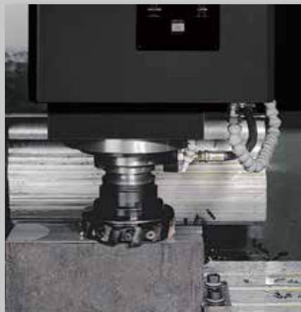
● Optimal Chip Removal (50#) Face Milling
