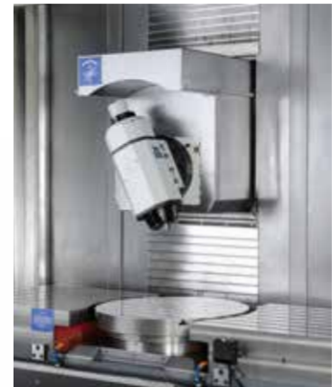
Big torque spindle 50kW, Swivel angle 120°, Rotation speed 33.3 rpm <TCV 3000A-5AX>(opt.)
