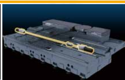
Centroid driven on X-axis to reduce vibration during movement, ensuring axial accuracy.<TCV 3000A-5AF / 5AX>
