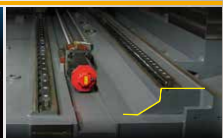
Stepped design on X-axis ensures stability during saddle movement. <TCV 3000A-5AF / 5AX>
