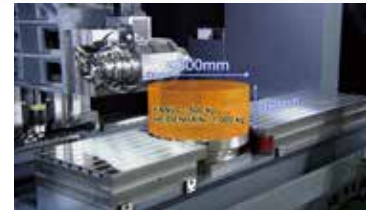
Resolution of rotary table: 0.001°
