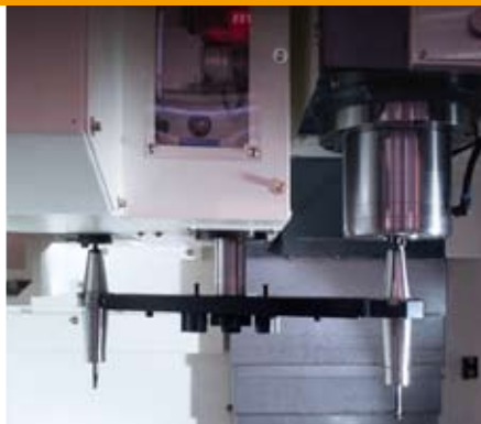
■ Auto Tool Change (T-T): 1.8 sec. IDD Spindle
